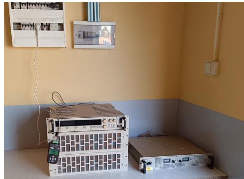
Electronic load and power supply (battery tests in laboratory)
