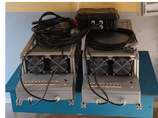
Handheld load bank (battery tests in the field)
